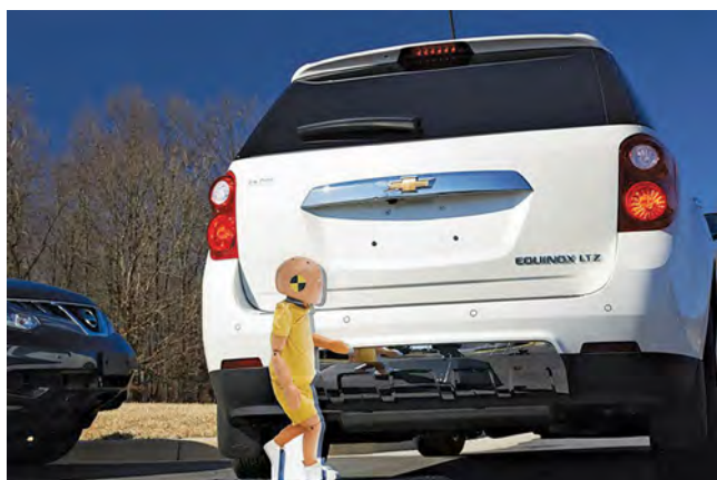
A foam cutout of a child is used in a rear end sensor test.
