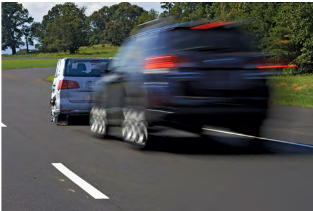
An inflatable car is used in a front end sensor test.
